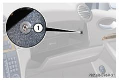
AUX socket: Socket for 3.5 mm stereo jack, for devices with dedicated analog audio output or connection via headphone port, e.g. MP3 or tape player
