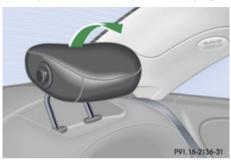
▶ Pull the head restraint forward until it locks into position.
